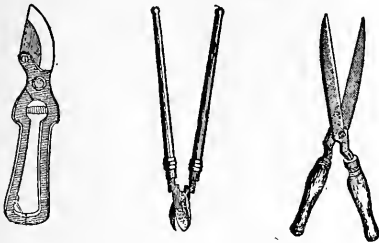
(a) Pruning shears; (b) lopping shears; (c) hedge shears. (L. C. Corbett.)
