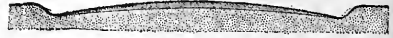
Cross section of road, showing clay cover on "deep" sand sub-soil. (Wm. L. Spoon.)
