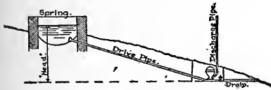
Setting of hydraulic ram. (E. T. Wilson.)
