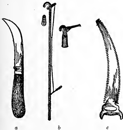
(a) The hawkbill knife; (b) device for cutting small limbs on tall trees; (c) double-edged curved-blade pruning saw. (L. C. Corbett.)
