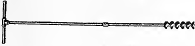
Soil auger for collecting soil samples and useful in exploring sub-soil conditions in lawns. Such an instrument entirely prevents the disfigurement which would be unavoidable if a larger hole had to be dug in a lawn. (L. C. Corbett.)
