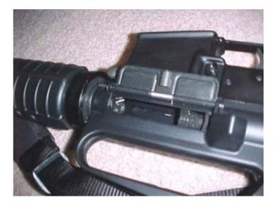
Next step once you are sure its empty, let the bolt go forward to you can take the rifle down, push lever in picture below and the bolt will close.
