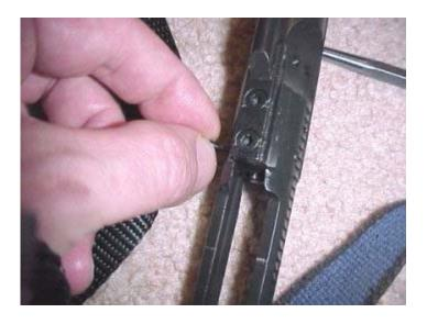
Tip the bolt on its back and the firing pin should come right out.
