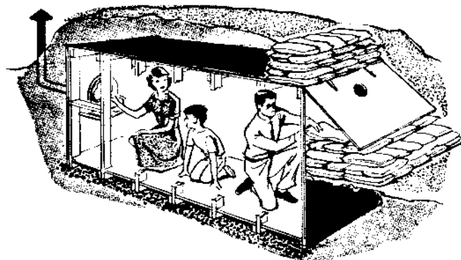
This backyard plywood shelter can be built partially above ground and mounded over with earth, or be built totally below ground level. A gravel drain under the shelter and a ditch outside help keep it dry. The family blocks the entrance with sandbags after entering the shelter.
