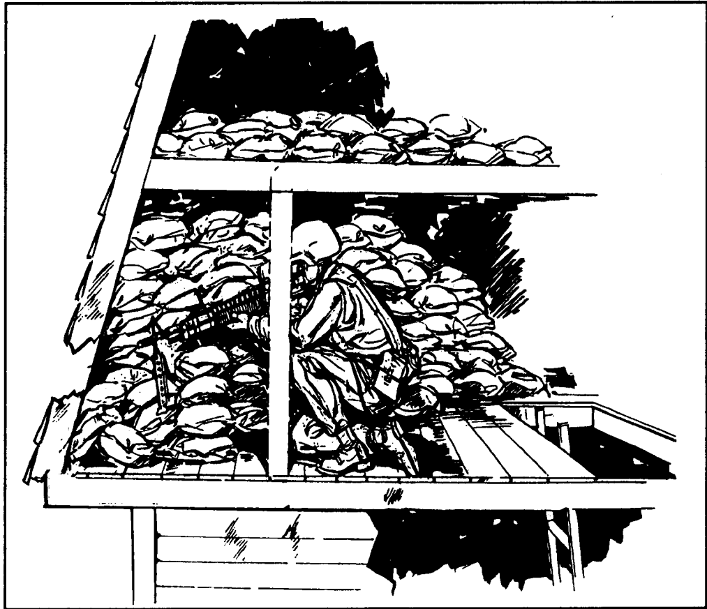
Figure 5-41. Firing platform built under roof.
