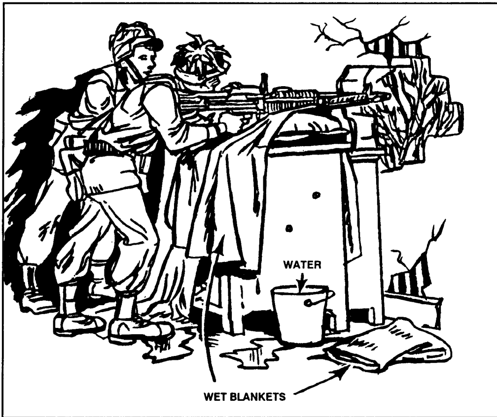
Figure 5-46. Wet blanket used to keep dust down.
