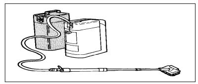
Figure A-8. M13 Decontaminating Apparatus, Portable
