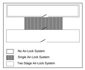
Figure B-2. Collective-Protection Entrance Configurations
