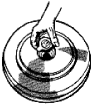
1 Removing Arming Plug From Mine.
