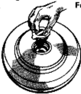
4 Inserting Arming Plug With Indicator At "SAFE" Position Into Mine Before Laying.
