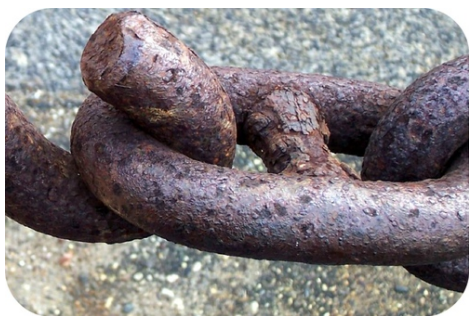
FIGURE 7: Rust (iron oxide) forms on an unprotected iron surface.
