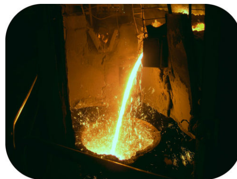
Molten (melted) iron is poured into a mold at a foundry. It takes extremely high temperatures to change iron from a solid to the liquid shown here. That's because iron has a very high melting point.
