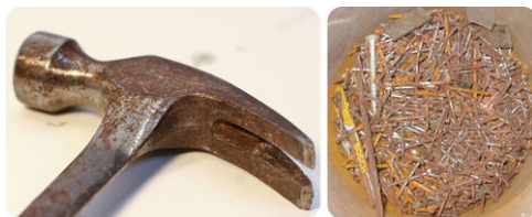
FIGURE 8: A rusting hammer, has a lower surface area than a pile of rusting nails.
