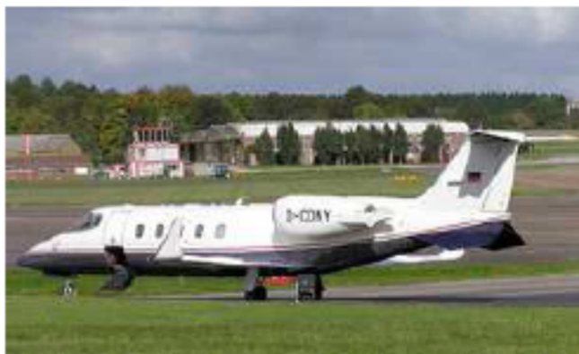
Figure C.10: “Fasten your cufflinks.” A Bombardier Learjet 60XR carrying 8 passengers at 780 km/h has a transport cost of 150 kWh per 100 passenger-km. Photograph by Adrian Pingstone.
