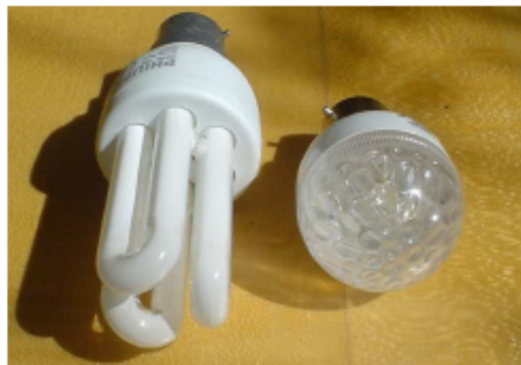
Figure 9.4: Philips 11W alongside Omicron 1.3W LED bulb.
