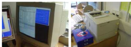
LCD CRT Printer: 17W 31W 108W (on, idle)
