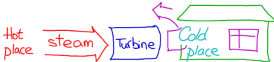
Figure 21.9: Combined heat and power. District heating absorbs heat that would have been chucked up a cooling tower.
