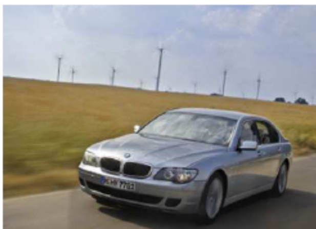
Figure 20.26: BMW Hydrogen 7. Energy consumption: 254 kWh per 100 km. Photo from BMW.
