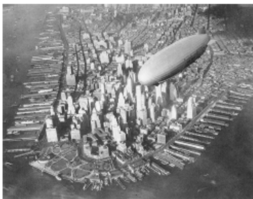
Figure C.14: The 239m-long USS Akron (ZRS-4) flying over Manhattan. It weighed 100 t and could carry 83 t. Its engines had a total power of 3.4 MW, and it could transport 89 personnel and a stack of weapons at 93 km/h. It was also used as an aircraft carrier.
