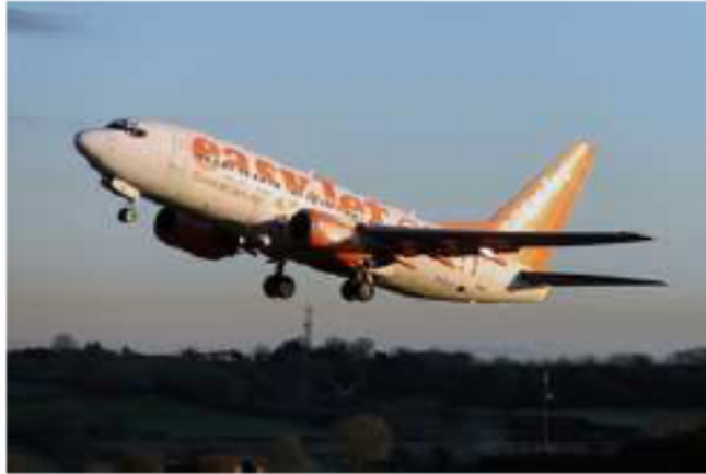
Figure C.11: Boeing 737-700: 30 kWh per 100 passenger-km. Photograph © Tom Collins.
