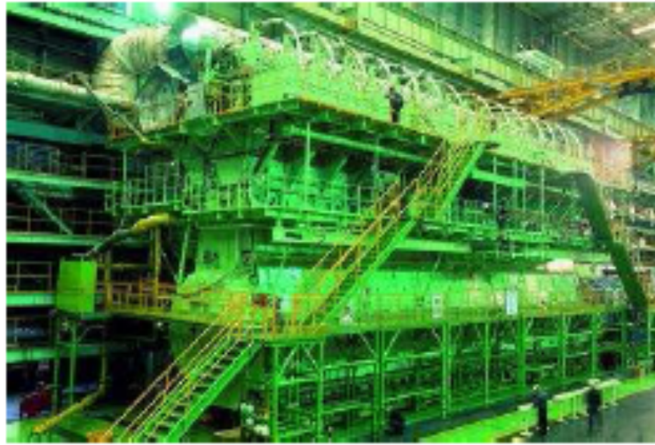
Figure A.15: The Wartsila-Sulzer RTA96-C 14-cylinder two-stroke diesel engine. 27m long and 13.5m high. www.wartsila.com
