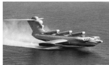
Figure C.16: The Lun ekranoplan – slightly longer and heavier than a Boeing 747. Photographs: A. Belyaev.
