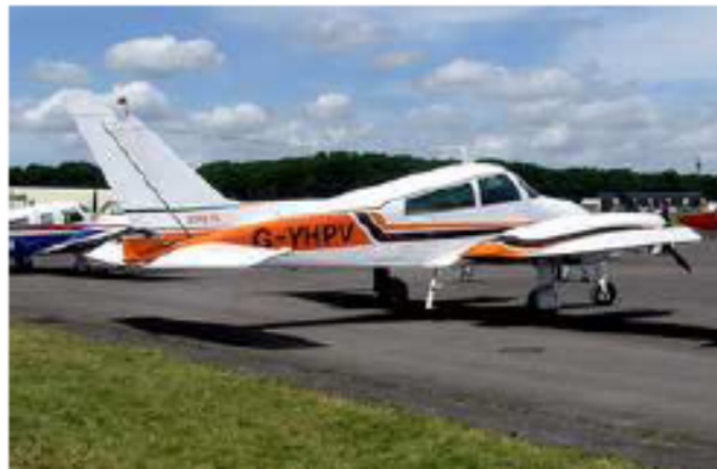
Figure C.9: Cessna 310N: 60 kWh per 100 passenger-km. A Cessna 310 Turbo carries 6 passengers (including 1 pilot) at a speed of 370 km/h. Photograph by Adrian Pingstone.
