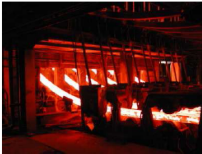
Figure H.1: Continuous casting of steel strands at Korea Iron and Steel Company.
