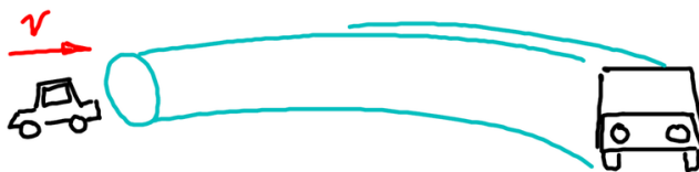
Figure A.3: A car moving at speed v creates behind it a tube of swirling air; the cross-sectional area of the tube is similar to the frontal area of the car, and the speed at which air in the tube swirls is roughly v .
