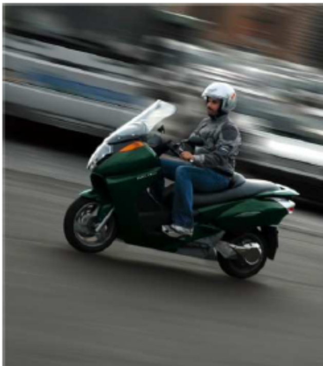
Figure 20.44: Vectrix: 2.75 kWh per 100 km. Photo from www.vectrix.com .
