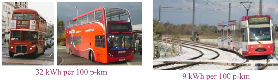
Figure 20.7: Some public transports, and their average energy consumptions. Left: Some red buses. Right: Croydon Tramlink. Photo by Stephen Parascandolo.
