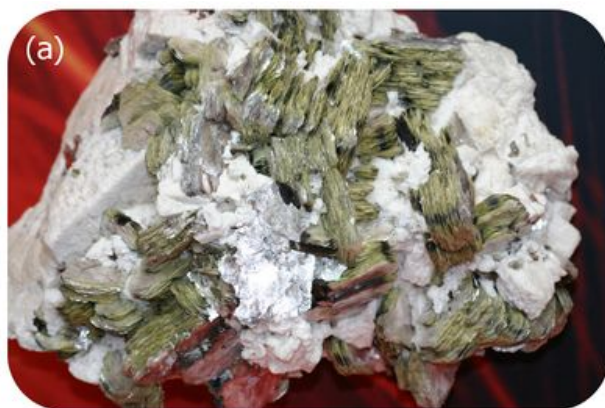
(a) Muscovite has platy cleavage due to the sheet-like structure of the silica tetrahedra.
