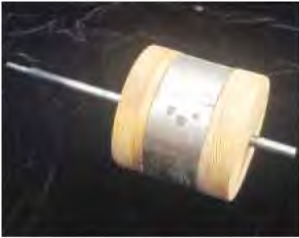
The wooden armature holds eight NdFeB (neodymium-iron-boron) magnets arranged in alternating polarity around its perimeter.
