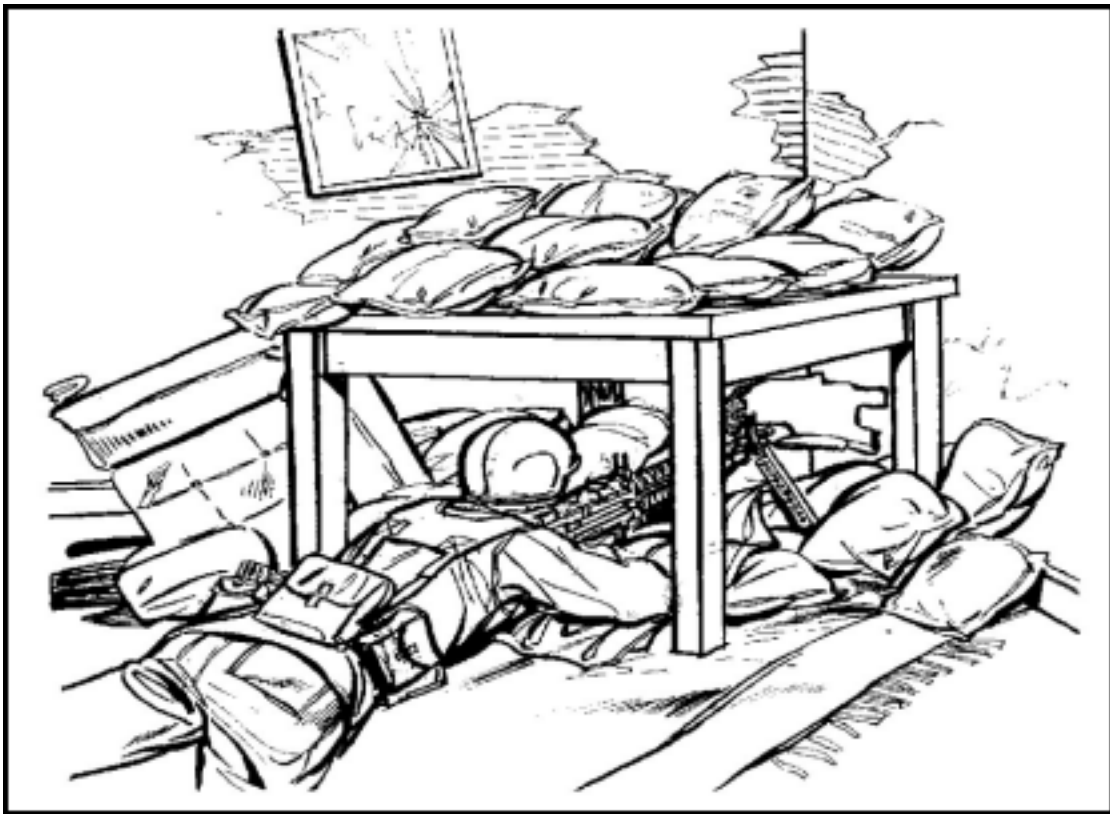
Figure 3-57. Corner machine gun bunker.
