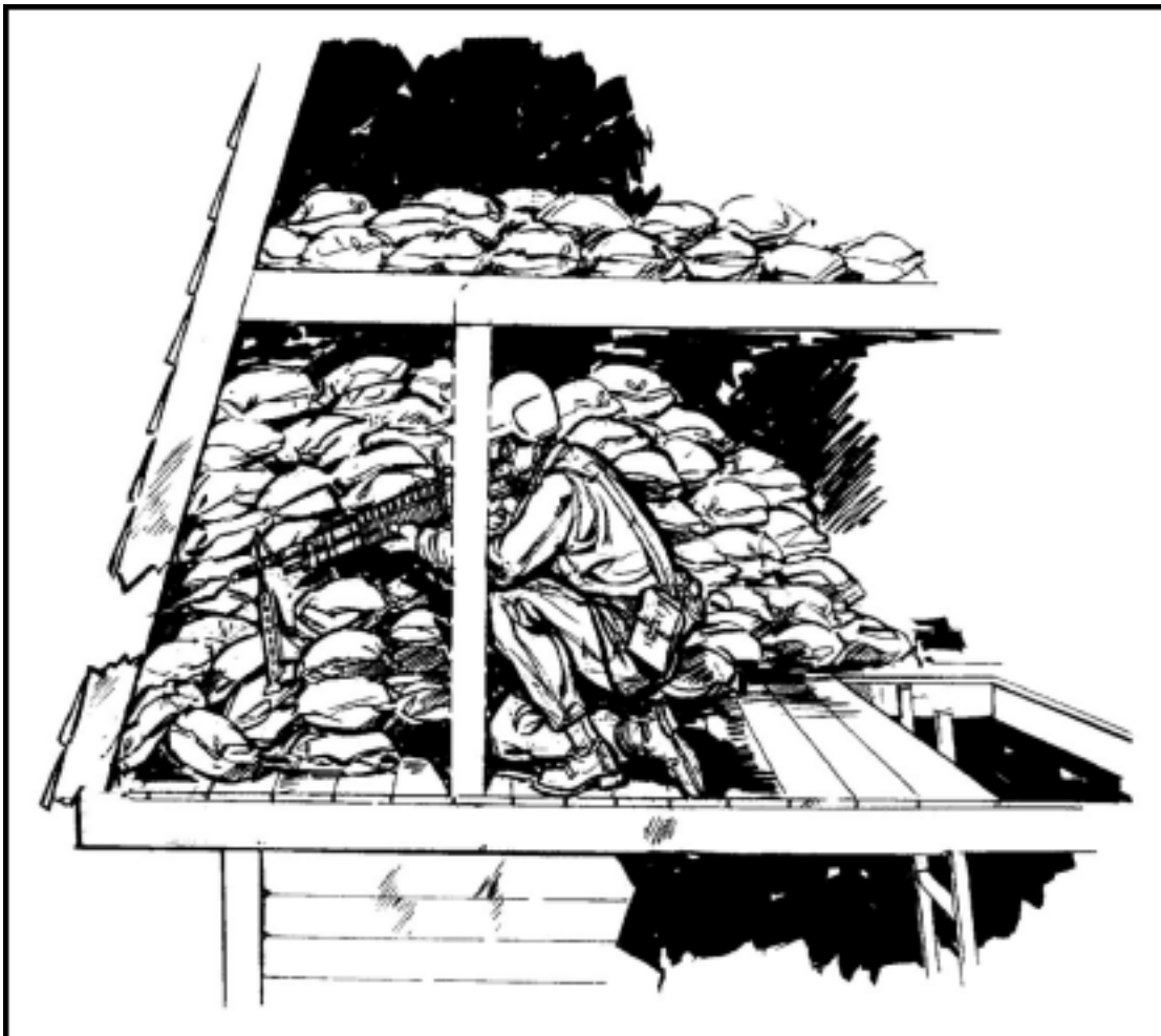
Figure 3-60. Firing platform built under roof.
