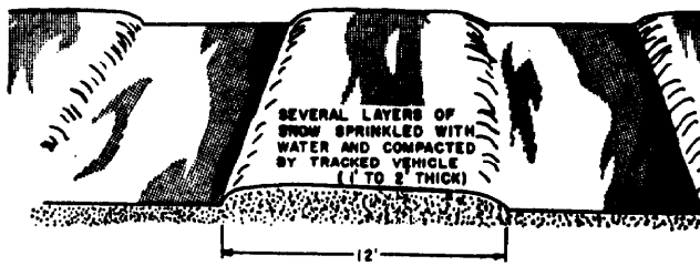
Figure 5-7. Road reinforced with snow.
