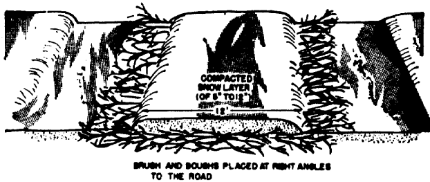
Figure 5-8. Road reinforced with brush and snow.
