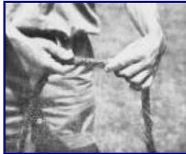
Testing the rope of bark fibre, breaking strain 1" [2.5 cm] diameter, about 800 lbs. [365 kg].
