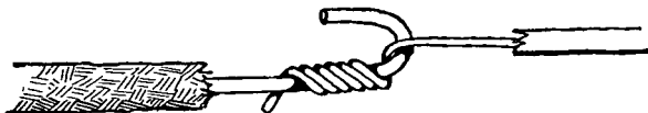
FIGURE 117.—A method of attaching connecting or detonating wire to a lead wire
