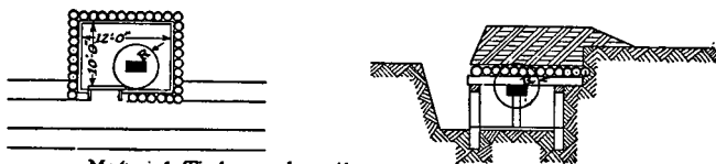
Material—Timber and earth. Charge—N·R 8 KC·25% R=3; K=0.375, C=4.5 N=(3)^2(375)(4.5) \cdot 25\% = 45.6 \cdot 11.4 N=57 blocks TNT Charge is supported against roof of shelter by struts
