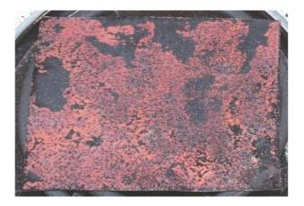
When the copper has cooled to room temperature (this takes about 20 minutes), most of the black oxide will be gone. A light scrubbing with your hands under running water will remove most of the small bits. Resist the temptation to remove all of the black spots by hard scrubbing or by flexing the soft copper. This might damage the delicate red cuprous oxide layer we need to make to solar cell work.
