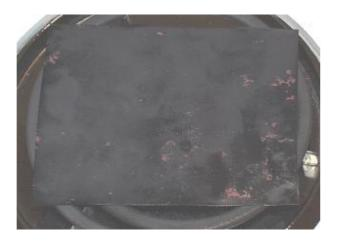
As the copper cools, it shrinks. The black cupric oxide also shrinks. But they shrink at different rates, which makes the black cupric oxide flake off.
