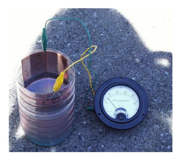
The photo above shows the solar cell in my shadow as I took the picture. Notice that the meter is reading about 6 microamps of current.
