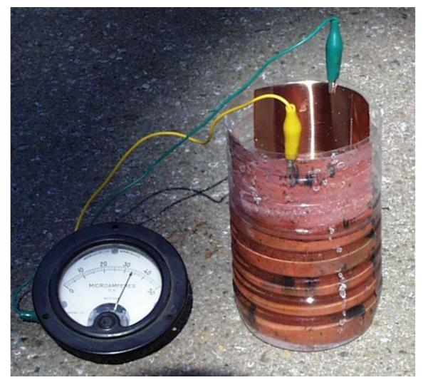
The above photo shows the solar cell in the sunshine. Notice that the meter has jumped up to about 33 microamps of current. Sometimes it will go over 50 microamps, swinging the needle all the way over to the right.
