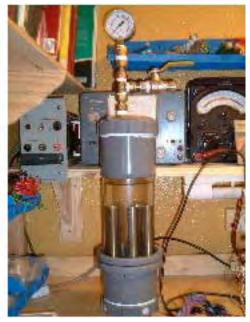
The electrolysis takes place between each of the inner and outer tubes. The picture above shows the bubbles just starting to leave the tubes after the power is switched on. The picture below shows the situation a few seconds later when the whole of the area above the tubes is so full of bubbles that it becomes completely opaque:
