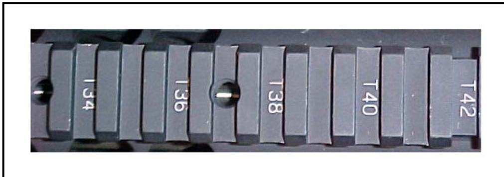
Figure 2-16. Address markings on RAS.
