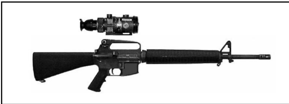
Figure 2-38. AN/PVS-4 on the M16A2-series weapons.
