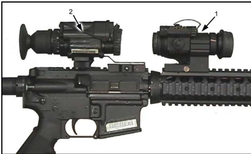
Figure 2-26. Mounting the M68/AN/PVS-14 combination on an MWS.
