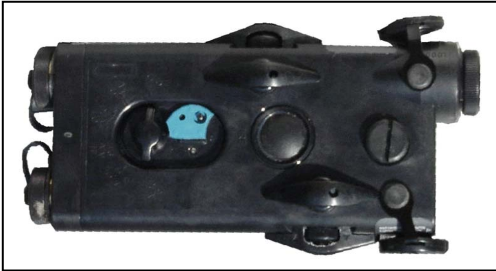
Figure 2-30. AN/PEQ-2A target pointer illuminator/aiming light.
