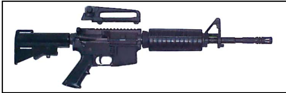
Figure 2-10. M4/M4A1 carbine with standard handguards installed.
