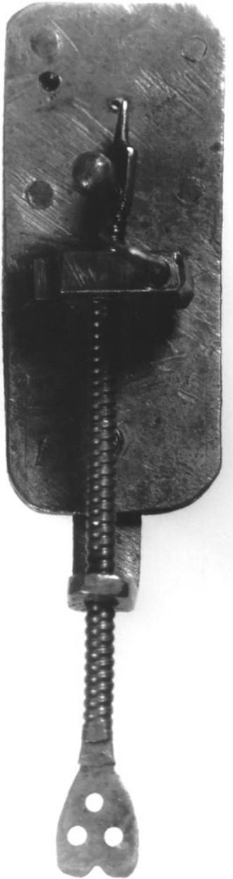
2.1 A van Leeuwenhoek microscope, one of the nine remaining microscopes known to be in existence.
