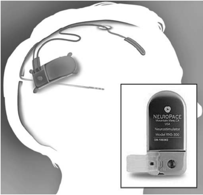
Figure 77.1 Schematic illustration of the implanted RNS Neurostimulator, depth lead and cortical strip lead. The RNS Neurostimulator (inset) is designed to match typical skull thickness and curvature, and is intended for implant in a ferrule, or socket, placed in a craniectomy. Up to two leads may be used with the system; each may be a depth lead or cortical (subdural) strip lead, and each has four electrode contacts, which are used for sensing and providing stimulation. In order to provide early seizure detection and delivery of focal electrical stimulation, leads are positioned using standard neurosurgical techniques as close as possible to the seizure focus or foci.
