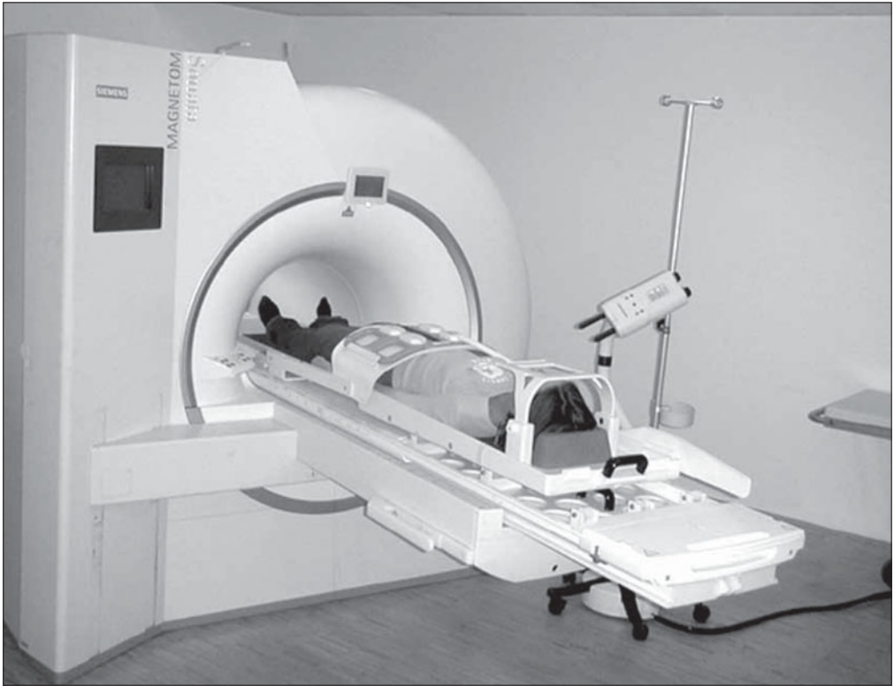
Figure 1.6 AngioSURF table platform (MR-Innovation GmbH, Essen, Germany) mounted on the examination table of a Siemens Sonata MR scanner with a patient lying on top. The table and coil position are shown for the third of five stations; for purposes of illustration, the table has been moved outside of the magnet: for the actual measurement the coil glider is positioned in the isocenter. For the MR whole-body examination, five contiguous 3D data sets are acquired from head to toe. The patient is moved manually on the platform between each data set. As the table is moved, the patient slides between a fixed RF receiver coil located posteriorly and a receiver coil mounted anteriorly on the coil glider. The glider follows the contour of the patient, which minimizes the separation of the coil to the patient, thereby optimizing the signal-to-noise ratio and the image quality. An additional frame protects the patient's face. The technique allows a fast MRI whole-body examination with high image quality (see Fig. 1.7).
