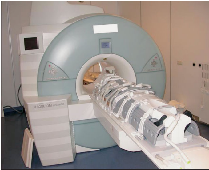
Figure 8.4 Patient in supine, head-first position. The patient is covered with several surface coils. The whole body can therefore be captured using parallel image acquisition in all three planes.
