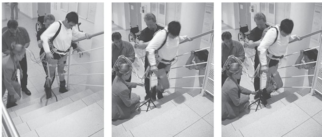
Figure 22.5. Paraplegic patient with a laboratory neuroprosthesis system applied to stair climbing (T. Fuhr, TU München). See also color insert.
