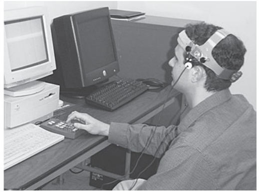
Figure 6.4. Transducer mounting designs: (left) elastic headband mounting bracket configured with a single transducer for unilateral recording; (right) welder's helmet mounting bracket affording bilateral recording capability.
