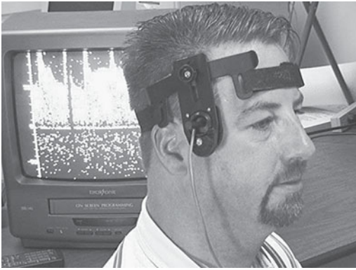
Figure 6.4. Transducer mounting designs: (left) elastic headband mounting bracket configured with a single transducer for unilateral recording; (right) welder's helmet mounting bracket affording bilateral recording capability.
