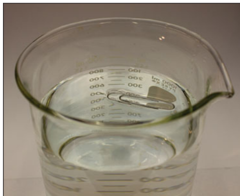
Figure 7.19 Surface Tension of Water
